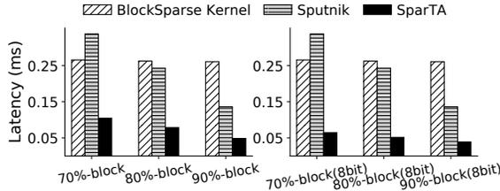
Figure 16: The performance of execution plan transformation for mixed sparsity patterns.  $B$  is sparsified for the matrix multiplication  $A \times B$  ( $1024 \times 1024 \times 1024$ ). “X%-block” means X% block sparsity mixed with 1% unstructured sparsity.
