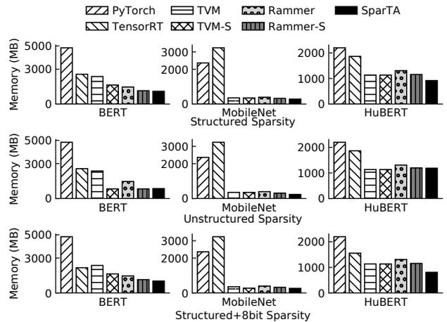
Figure 9: GPU memory usage of different models with three sparsity patterns on NVIDIA 2080 Ti.
