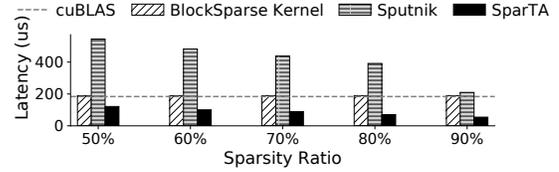
Figure 17: The performance of execution plan transformation leveraging Sparse Tensor Cores.  $B$  is sparsified with different sparsity ratios for  $A \times B$  ( $1024 \times 1024 \times 1024$ ).
