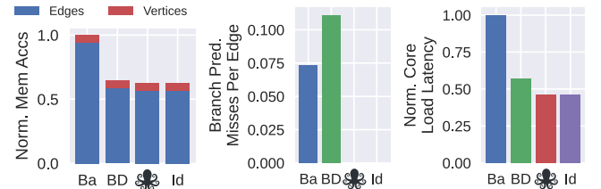
Figure 17: HATS performance breakdown. Left: DRAM accesses split by PageRank phase. Mid: core branch mispredictions per graph edge processed. Right: cumulative core load latency.
